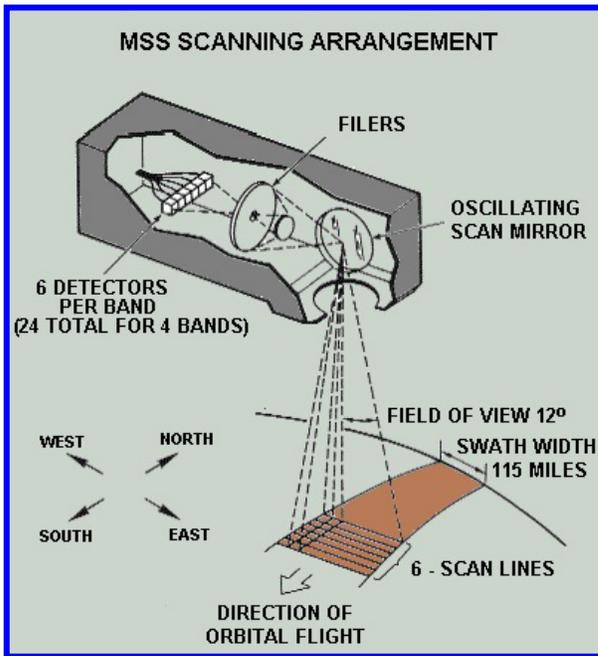
**FIGURE 7: Multispectral Scanner System**
