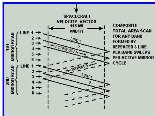
**FIGURE 8: Scan Track Direction**
